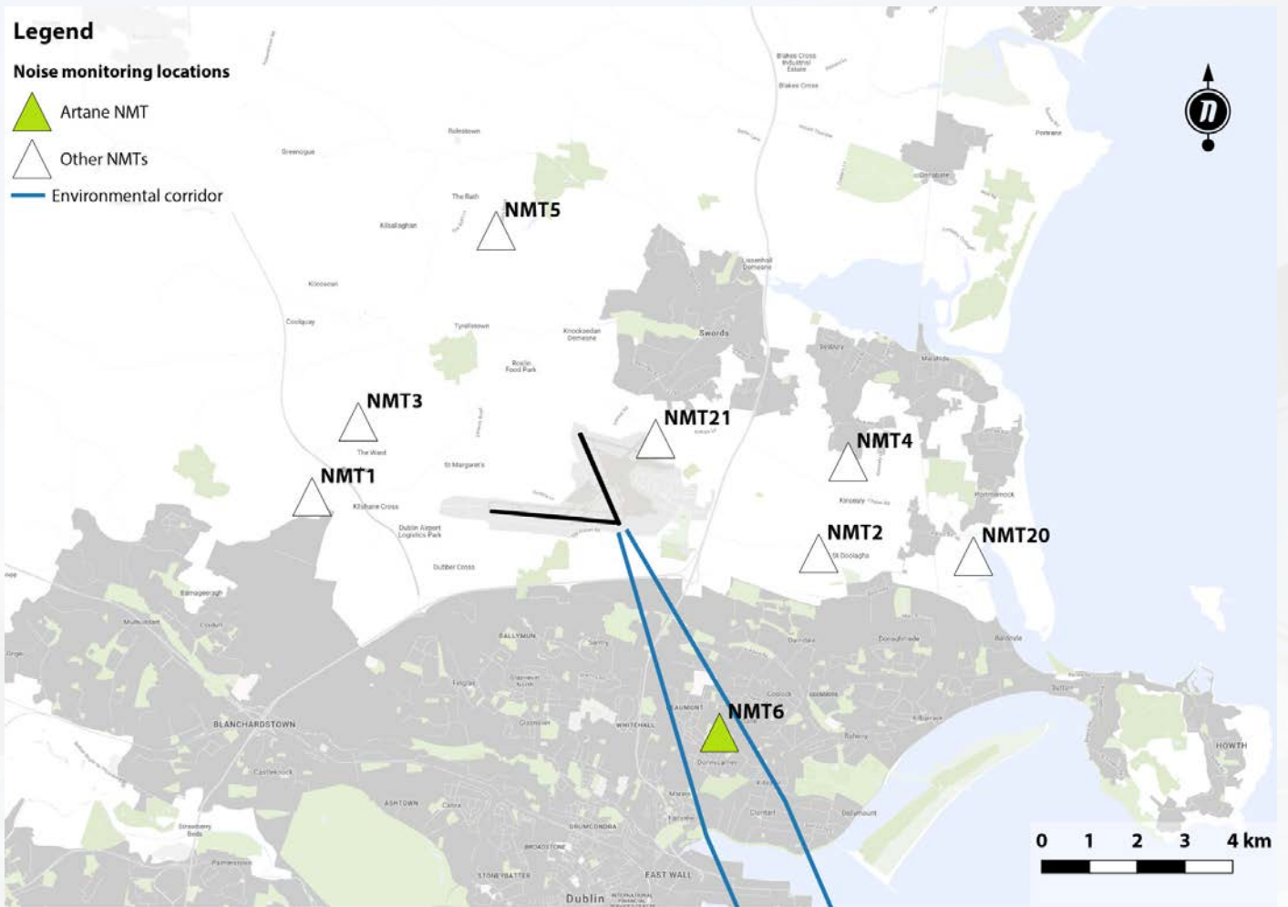
Figure 34: Noise Monitoring Terminal Artane Location
